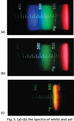
Fig. 5. (a)-(b) the spectra of white and yellow glowing RGB light mixer and (c) the spectrum of yellow LED. The scale shows the wavelength in nm.
