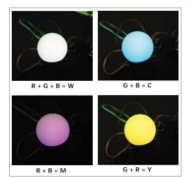
Fig. 2. Combining red (R), green (G), and blue (B) lights with the ball light mixer, white (W), cyan (C), magenta (M), and yellow (Y) color can be produced.
